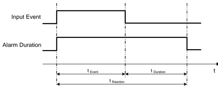
**t<sub>Event</sub>:** Duration of alarm input source (motion, contact, system events...)
