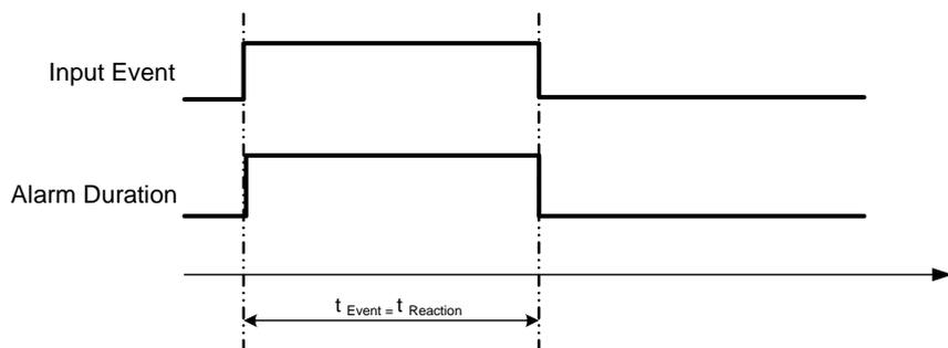
**t<sub>Event</sub>:** Duration of alarm input source (motion, contact, system events...)
