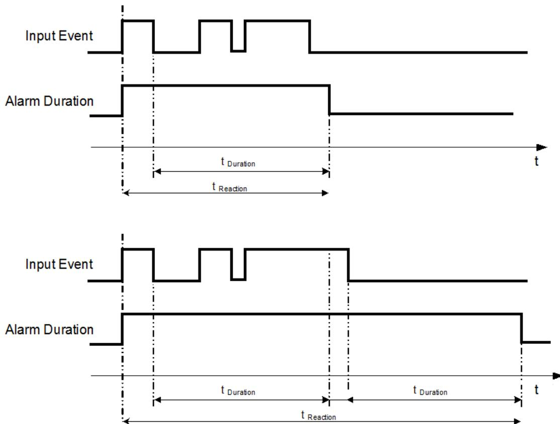
**t<sub>Event</sub>:** Duration of alarm input source (motion, contact, system events...)
