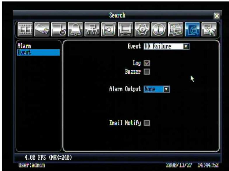
Figure 5.15 (Alarm & Event Menu – Event - HD Failure)
