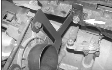
17. Using the battery tray mounting bolt that was removed in step 15, mount the throttle body bracket to the battery tray as shown.
