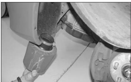
30. From underneath the vehicle, install the K&N Filtercharger onto the K&N intake tube.
