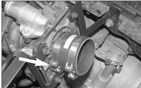
19. Install the supplied silicone hose and hose clamps to the throttle body and tighten throttle body hose clamp.
