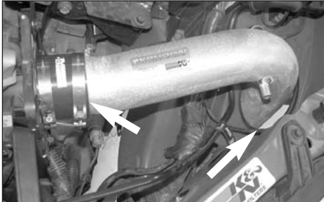
23. Slide the K&N intake tube down the resonator hole then insert the other end into the throttle body silicone hose.
