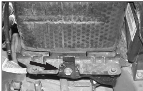
15. Remove the battery tray mounting bolt. This bolt will be re-used.
