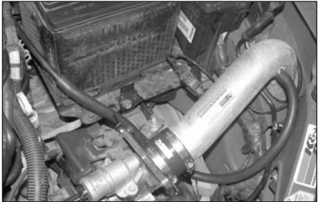
28. Using the supplied silicone hose, attach one end to the K&N intake tube and the other end to the crankcase vent tube.
