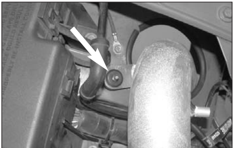
24. Align the K&N intake tube bracket to the stock airbox mount.
