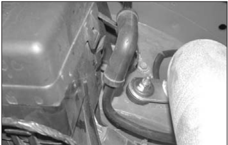
25. Using the supplied nut, tighten the intake tube bracket to the stock stud.
