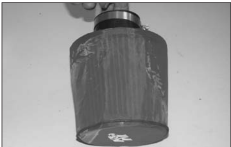
29. Install the K&N Drycharger and hose clamp onto the K&N Filtercharger.
