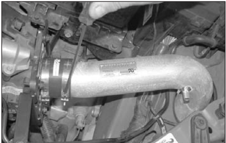
26. Align the intake tube and tighten throttle body hose clamp.
