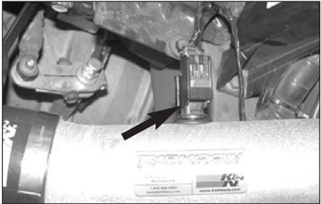
27. Install the air temp. sensor into the rubber grommet on the K&N intake tube.
