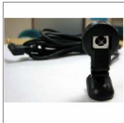
IR extender is designed to extend the IR receiver which is allowed to be used on 4/8ch Triplex DVR.
