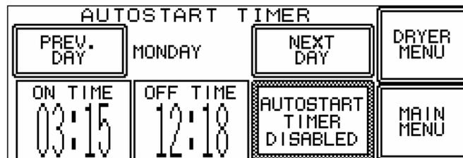
This screen allows the operator to set the time and day that the dryer will start **automatically**. Reference page 32, Make sure the clock is set to current date and time.
