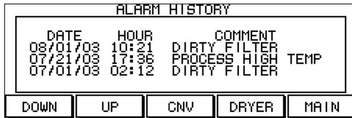
This screen allows the operator to review the number and type of issues that the Drying/Conveying System has encountered during its operation.
