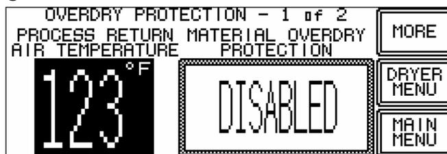
The **PROCESS RETURN AIR TEMPERATURE** displays the air temperature as it leaves the drying hopper. If this temperature is above 150°F, an aftercooler is required.
