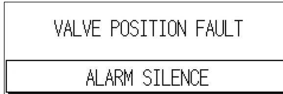
This is an example of what a typical Alarm screen looks like. The user will see the message causing the alarm in the top half of the display with an **ALARM SILENCE** button in the lower half.
