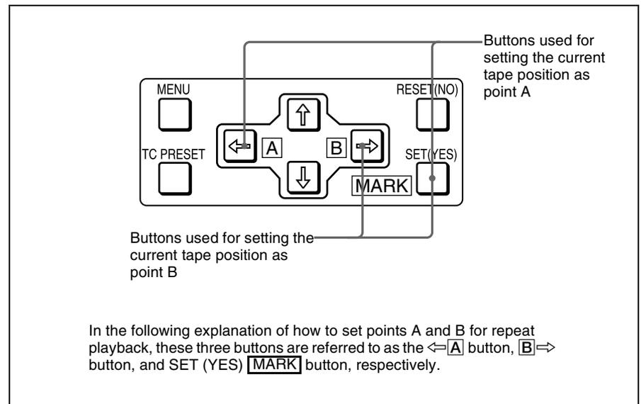
While holding down the SET (YES) **MARK** button on the menu control panel, press the **A** or **B** button. The time code value of the current tape position is set as point A or B, and a message “A set” or “B set” is displayed for 0.5 second in the time counter display.
