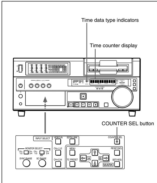
Open the door on the lower part of the front panel, and press the COUNTER SEL button. Each press of this button cycles through three options: CNT value, time code, and user bit data. The time data type indicator for each option lights as it is selected.
