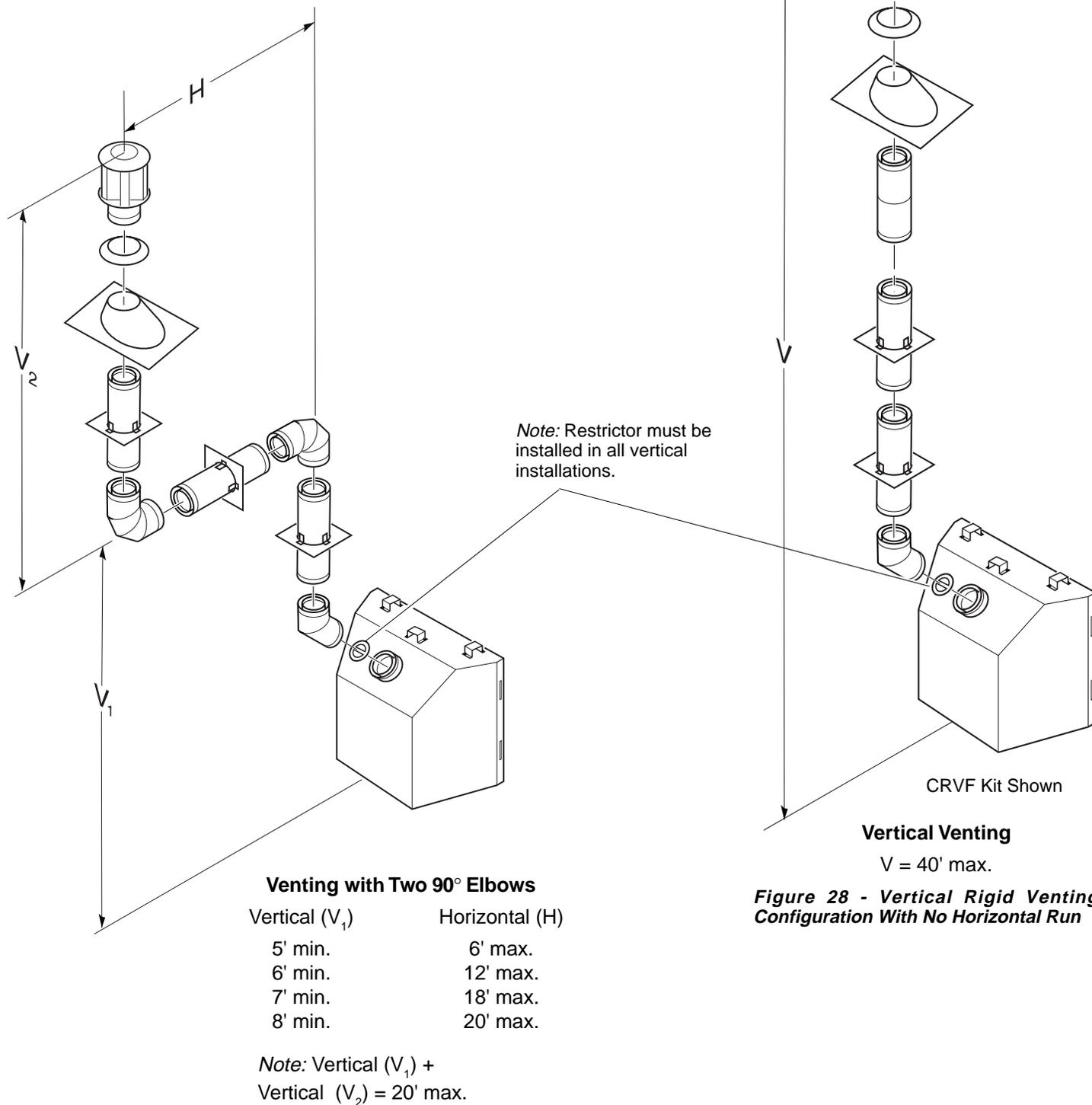
Figure 27 - Vertical Rigid Venting Configuration Using Two 90° Elbows
