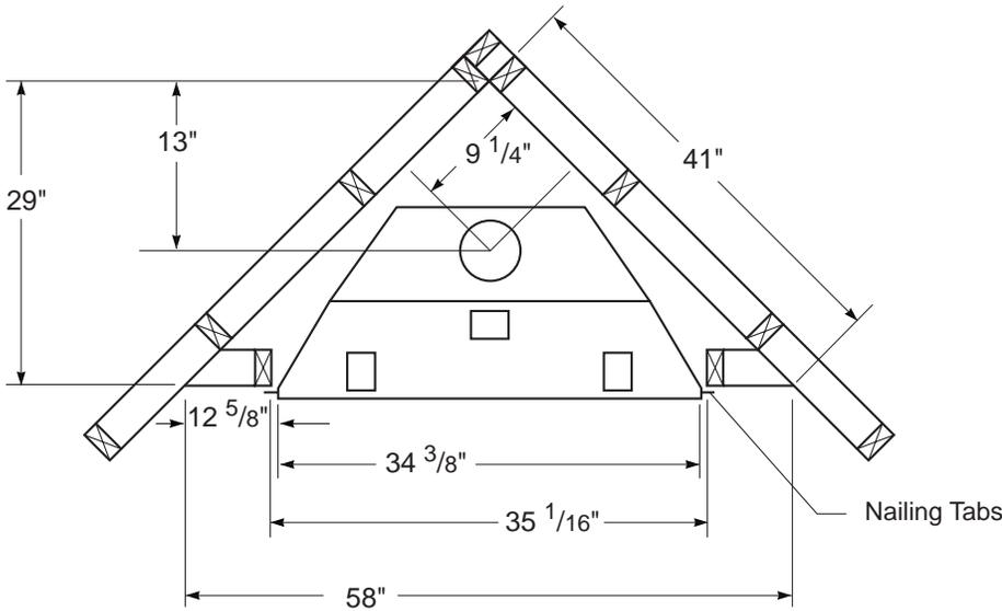
**Figure 6 - Framing Clearances for Corner Installation**
