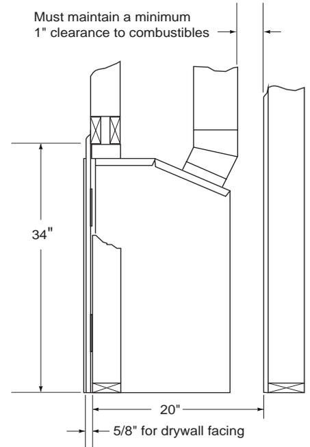
Figure 5 - Framing Clearances for Typical Fireplace Installation
