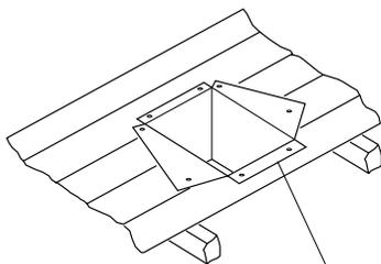
**Figure 24 - Installed Cathedral Ceiling Support Box**
