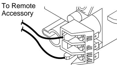
**Figure 41 - Connecting Remote Accessories to Control Valve**
