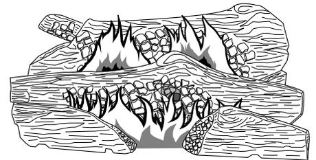
**Figure 55 - Typical Flame Pattern for CDV34NA, PA**
