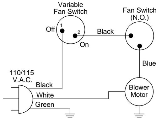
Figure 56 - Blower Wiring Diagram for Thermostat-Controlled Models
