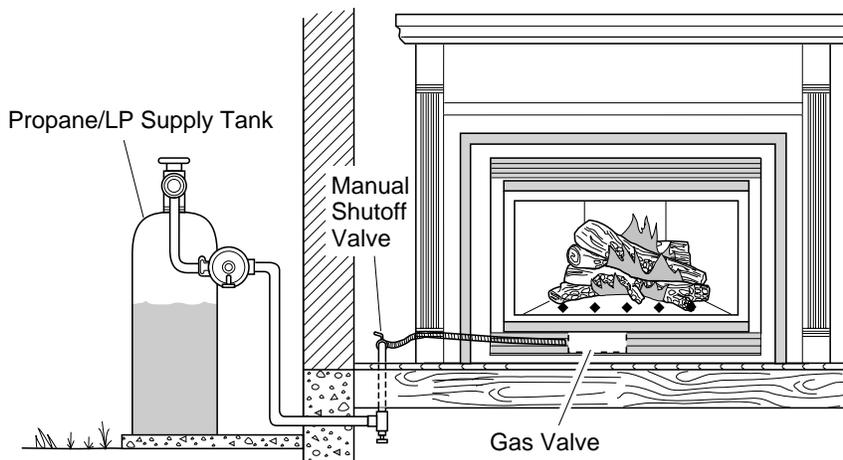
**Figure 38 - Checking Gas Joints for Propane/LP Gas Fireplace**
