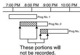
If the starting and ending times of two or more timer recordings overlap on the same day, priority is given to the earliest recording. For example, in the diagram at left **PROGRAM 2** will not be recorded until **PROGRAM 1** is finished. The first part of **PROGRAM 2** will not be recorded. Likewise, **PROGRAM 3** will not be recorded until **PROGRAM 2** is finished, and so on.
