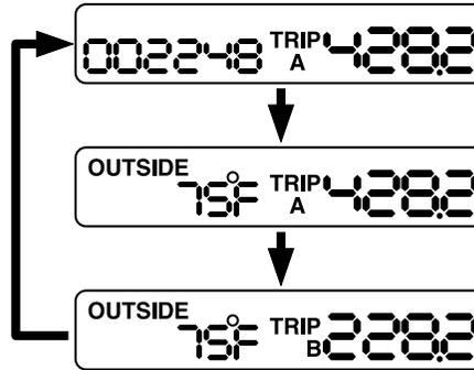
The temperature sensor is located in the front bumper. Therefore, the temperature reading can be affected by heat reflection from the road surface, engine heat, and the exhaust from surrounding traffic. This can cause an incorrect temperature reading when your speed is under 19 mph.
