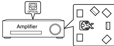
The recorder outputs digital audio signals in the bitstream format when you play a DVD video disc recorded on the Dolby Digital, DTS, MPEG1 and MPEG2 recording system.
