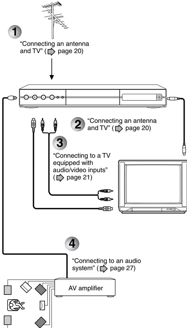
■ **When you connect a TV equipped with audio/video inputs**
