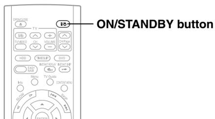
When the power turns on, ON/STANDBY indicator changes color from red (standby mode) to green (operation).
