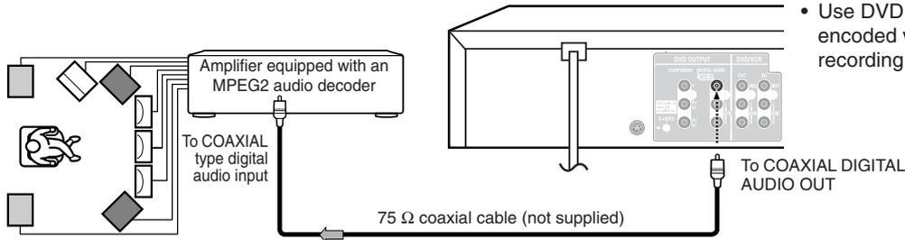
**Connecting to an amplifier equipped with a digital audio input**
