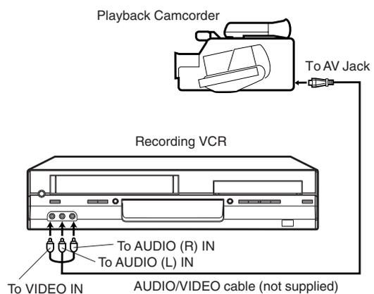
For duplicating a previously recorded tape from a camcorder, follow the camcorder manufacturer's instructions. A typical camcorder dubbing hookup is shown above.
