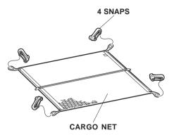
2. Attach the four snaps of the cargo net to the four tie-down hooks.
