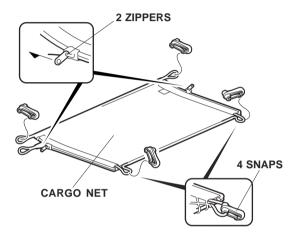
3. Attach the upper two loops on the cargo net to the two anchors. Then attach the two snaps on the cargo net to the two loops as shown.
