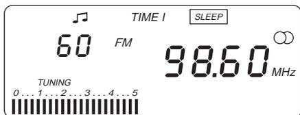
Repeated pressures on the  SLEEP button will reduce the switch-on period in steps of 10 minutes.
