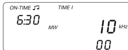
When activating the automatic tuning mode, the unit automatically switches to the higher tuning step. However, the 9 kHz or 10 kHz choice in the MW band is retained.
