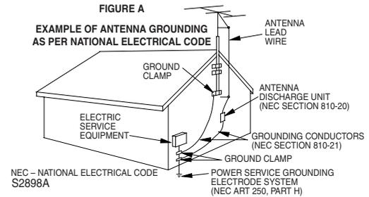
14. Lightning - For added protection for this video product during a lightning storm, or when it is left unattended and unused for long periods of time, unplug it from the wall outlet and disconnect the antenna or cable system. This will prevent damage to the video product due to lightning and power-line surges.
