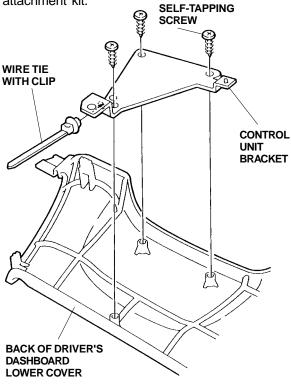
22. Position the control unit on the control unit bracket, and install the two 4 x 30 mm washer-screws. Secure the antenna to the control unit bracket with the wire tie with clip you just installed, as shown. Secure the antenna parallel with the control unit.
