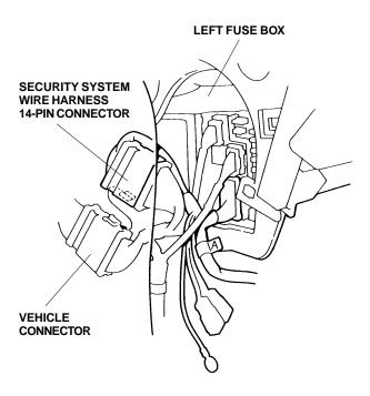
27. Locate the two 2-pin connectors blue-taped to the vehicle harness, and remove the blue tapes to free the connectors. Plug the 2-pin connectors you just freed into the 2-pin connectors of the security system wire harness. Connect the blue 2-pin connector of the vehicle harness to the blue 2-pin connector of the security system wire harness.
