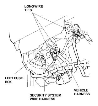
42. On the left of the fuse box, secure the security system wire harness to the vehicle harness with two long wire ties.
