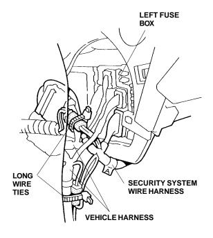
43. Plug the 3-pin connector of the security system wire harness into the 3-pin connector of the disarm switch harness. Plug the 22-pin connector of the security system wire harness into the control unit; then reinstall the driver's dashboard lower cover.
