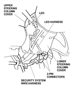
40. Secure the security system wire harness and the LED 2-pin connector to the vehicle harness with three long wire ties and one short wire tie. Secure the wire ties only in the areas shown and not to the yellow SRS harness.
