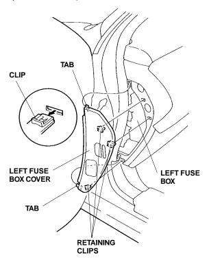
6. Remove the driver's dashboard lower cover (three screws, and five retaining clips).
