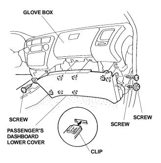
Open the glove box, and remove the two screw caps and seven self-tapping screws. Unplug the connector, and remove the glove box by pulling it toward you.
