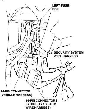
26. Attach the 14-pin connector of the security system wire harness to the side of the vehicle connector.
