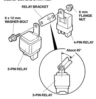
38. Plug the 6-pin and 4-pin connectors of the security system wire harness into the 5-pin and 4-pin relays; then attach the relay bracket to the steering hanger beam with one 6 x 12 mm washer-bolt and 6 mm flange nut. (The 5-pin relay has a 6-pin connector.)
