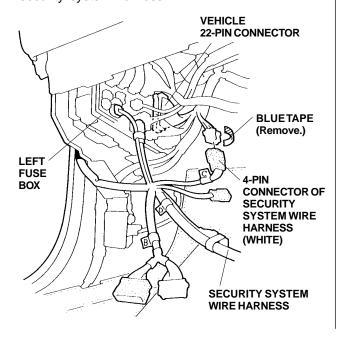
31. Unplug the 20-pin connector from the left fuse box, and plug the two 20-pin connectors (white) of the security system wire harness in between.
