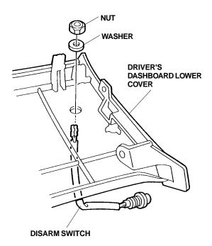
20. Locate the 3-pin connector included in the kit. Firmly push the disarm switch terminals into the 3-pin connector until they click into position, and lower the lock. Slide the white connector clip onto the underside of the 3-pin connector.
