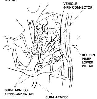
45. Push the clip of the sub-harness 4-pin connector into the hole in the right front inner lower pillar.
