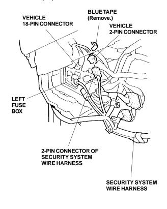
33. Remove the clip from the hole in the left knee bolster, use a utility knife to cut the clip off of the vehicle harness. Take care not to damage the vehicle harness.
