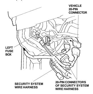
32. Locate the 2-pin connector blue-taped to the vehicle harness 18-pin connector, and remove the blue tape to free the connector. Connect the 2-pin connector you just freed to the 2-pin connector of the security system wire harness.
