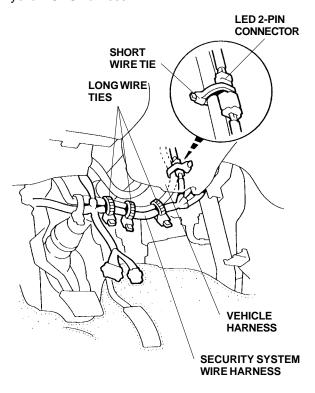
41. On the left of the steering wheel, secure the security system wire harness to the vehicle harness with three long wire ties in the areas shown.
