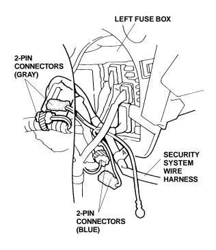
28. Remove the upper bolt that fastens the engine hood opener, and attach the ground terminal of the security system wire harness with the ground bolt from the kit.
