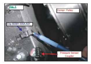
40. Install the other receiver pipe clip from the kit into the hole in the ABS bracket.
