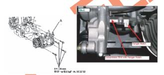
35. Get the discharge hose from the kit. At the front right side of the vehicle, route the hose end of the discharge hose on the right side of the radiator and to the compressor. Remove the 6 mm nut and the discharge port cover from the compressor. Discard the port cover, but save the 6 mm nut. Remove the pipe cover from the end of the discharge hose, and attach the discharge hose to the compressor, reusing the M6 nut.
