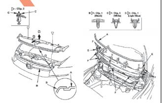
27. Remove the front bumper, two screws and twleve clips.
