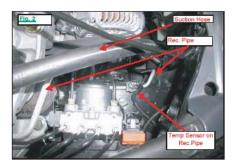
47. Remove the cap from the expansion valve. Get the stud bolt from the kit, and secure its short M6 side to the expansion valve.
