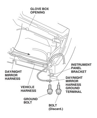
34. Remove and discard the instrument panel bracket bolt, and secure the day/night mirror harness ground terminal to the instrument panel bracket with the new ground bolt supplied. 35. Tape a piece of steel wire to the 4-pin connector end of the day/night mirror harness. Route the harness end up along the instrument panel side bracket, and out through the clearance between the right front pillar and the instrument panel as shown.
