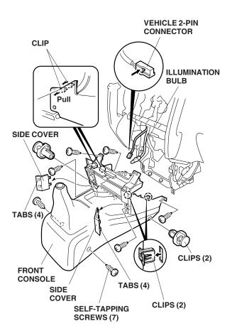
22. On M/T vehicles only, remove the two clips and seven self-tapping screws, and pull the front console out toward you to release four clips. Unplug the vehicle 2-pin connector from the accessory socket, then remove the front console. 23. Slide the day/night mirror stay onto the mirror holder, then tighten the T20 Torx screw installed on the day/night mirror.
