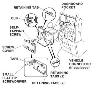
17. Remove two self-tapping screws that fasten the heater A/C control panel to the dashboard. Pull the heater A/C control panel out toward you to release the four clips. Unplug the vehicle connector, and remove the heater A/C control panel.
