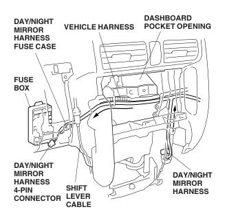
32. Connect the day/night mirror harness 4-pin connector to the accessory terminal of the fuse box.
