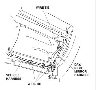
43. Secure the day/night mirror harness to the vehicle harness with three wire ties.
