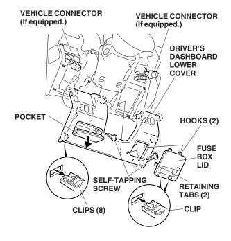
16. Open the dashboard pocket lid. Using a flat-tip screwdriver wrapped with tape, remove the screw cover by releasing the two retaining clips and two retaining tabs. Remove the dashboard pocket (one self-tapping screw, then pull out to release the one clip and three retaining tabs). If equipped, unplug the vehicle connector.
