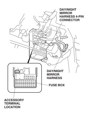
33. Route the day/night mirror harness ground terminal to the right along the vehicle harness at the rear of the glove box frame.
