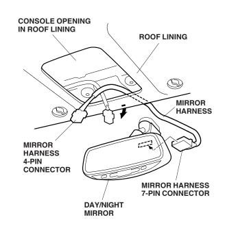
25. Route the mirror harness through the grooves of the upper and lower covers. Attach the lower cover to the stay of the mirror.
