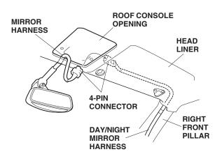
Connect the day/night mirror harness 4-pin connector to the mirror harness 4-pin connector. 39. Secure the three clips from the day/night mirror harness into the holes in the right front pillar.
