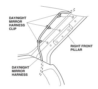
40. Using isopropyl alcohol, clean the areas where the cushion tapes will attach. Using scissors, cut two EPT sealers in half. Secure the day/night mirror harness to the roof panel with three EPT sealers.
