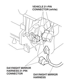
29. Remove the connector clip from the vehicle 21-pin connector (white) and install the new clip supplied with the kit onto the vehicle 21-pin connector.
