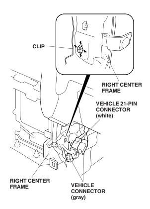
28. Unplug the vehicle 21-pin connector (white) and connect the day/night mirror harness 21-pin connectors between the vehicle 21-pin connectors (white).
