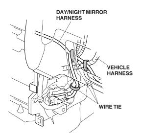
44. Under the dashboard, secure the day/night mirror harness to the vehicle harness with three wire ties.
