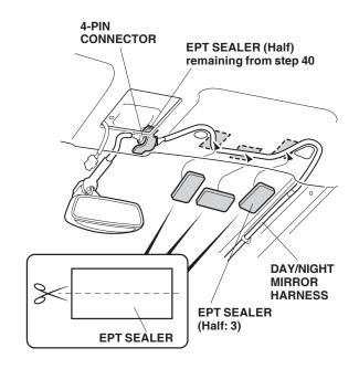
41. Using the remaining half of EPT sealer, secure day/night mirror harness 4-pin connector to the roof panel.
