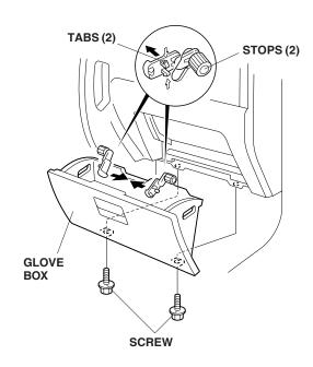
12. Remove the two screws from the bottom of the glove box, and remove the glove box.
