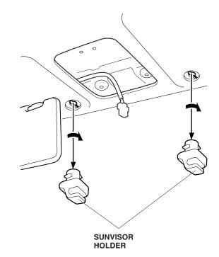
7. Remove the cap from the right sunvisor (four retaining tabs).
