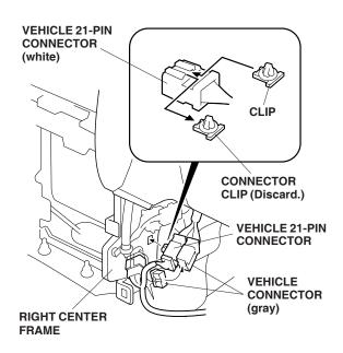
30. Reconnect the vehicle connector (gray) and attach the clip you just installed on the vehicle 21-pin connector (white) to the right center frame.
