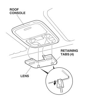
4. Remove the roof console (four screws, and unplug one connector).
