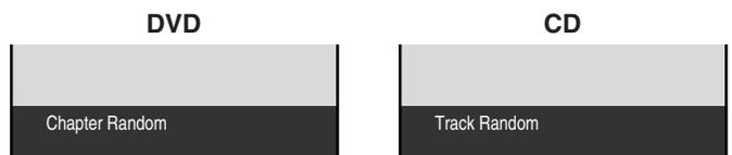
2 During playback random playback will start automatically. To start random playback during stop mode, press **▶** within about 5 seconds after you press the **PLAY MODE**.
