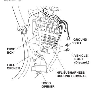
17. Disconnect the vehicle harness 1-pin connector and connect it to the HFL subharness 1-pin connector.
