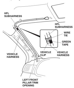
15. Route the HFL subharness and secure the harness to the vehicle harness with a wire tie above the vehicle clip as shown.
