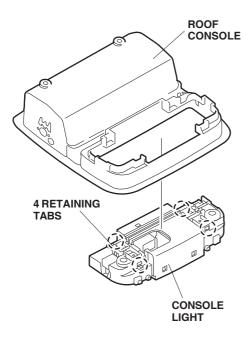
28. Enlarge the hole on the roof console with 9 mm drill bit.
