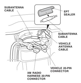
23. Plug the vehicle antenna cable into the subantenna cable.
