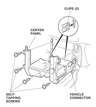
7. If equipped with a cigarette lighter, remove the four self-tapping screws. Pull the center panel by releasing the two clips. Unplug the two lighter harness terminals, and remove the illumination light. Remove the center panel.
