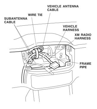
24. Secure the XM radio harness and subantenna cables to the vehicle harness with a wire tie.
