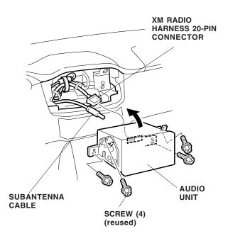
29. Secure the XM radio harness, subantenna cables, and display module cable to the vehicle pipe with two wire ties.
