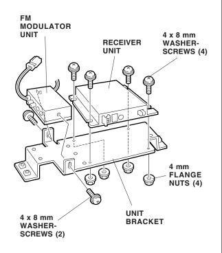
49. Install the FM modulator unit tn the unit bracket with the two 4 x 8 mm washer-screws.
