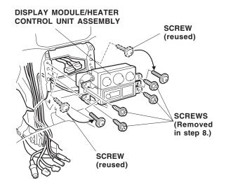
28. Plug the XM radio harness 20-pin connector and sub antenna cable into the audio unit, and carefully slide the audio unit into the dashboard. Reinstall the four audio unit screws.
