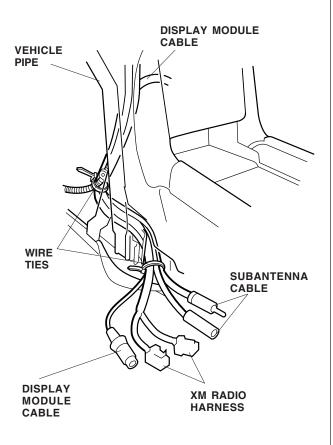
30. Continue routing cables through the center console and toward the rear of the vehicle. Using scissors, cut one cushion tape in half. Clean the vehicle frame with isopropyl alcohol, and attach half of the cushion tape to the vehicle frame in the area shown.
