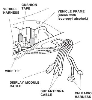
32. Attach the remaining half of the cushion tape to the vehicle frame in the area shown.
