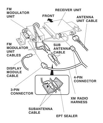
52. Wrap one EPT sealer around the subantenna cables.
