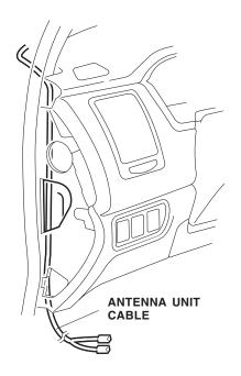
45. Secure the antenna unit cable to the vehicle harness with two wire ties.
