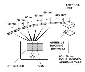
40. Using isopropyl alcohol on a shop towel, clean the bottom of the antenna unit. Remove the backing from the 60 x 60 mm double-sided adhesive tape, and attach it to the bottom of the antenna unit.
