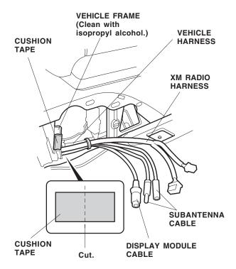
31. Secure the XM radio harness and subantenna cables with one wire tie, but don't tighten the wire tie at this time.
