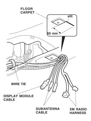
34. Route the XM radio harness and subantenna cables under the floor carpet and out the slit. Secure the cables with one wire tie.
