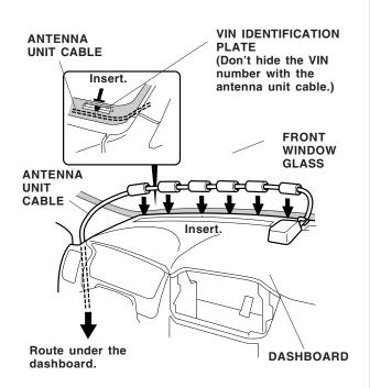
44. Route the antenna unit cable down and under the dashboard.
