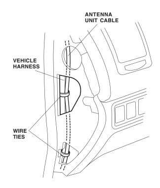
46. Below the dashboard, secure the antenna unit cable to the vehicle harness with two additional wire ties.
