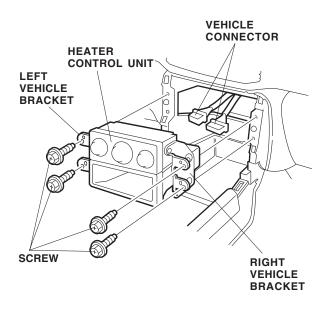
9. Remove the left and right vehicle brackets (six self-tapping screws), and separate the heater control unit from pocket. Set the pocket aside, it will not be reused.
