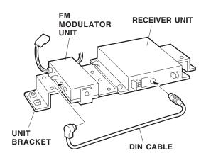
51. Position the unit assembly under the driver's seat. Plug the XM radio harness 4-pin connector and the antenna unit cables into the receiver unit. Plug the XM radio harness 3-pin connector, the display module cable, and the subantenna cables into the FM modulator unit.
