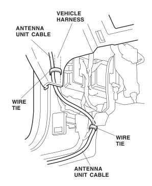
47. Continue routing the antenna unit cable alongside the vehicle harness, and out through the hole in the floor carpet under the driver's seat. Secure the antenna unit cable to the vehicle harness with four wire ties in the area shown.
