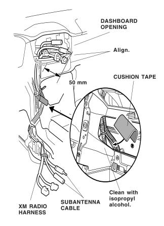
21. Pull the XM radio harness and subantenna cables out through the dashboard opening approximately 50 mm.
