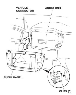
4. Remove the four screws that fasten the audio bracket. Pull the audio unit out toward you, and unplug the vehicle connector and antenna cable from the rear of the audio unit. If equipped with a cassette/in-dash CD changer, unplug the additional connectors.
