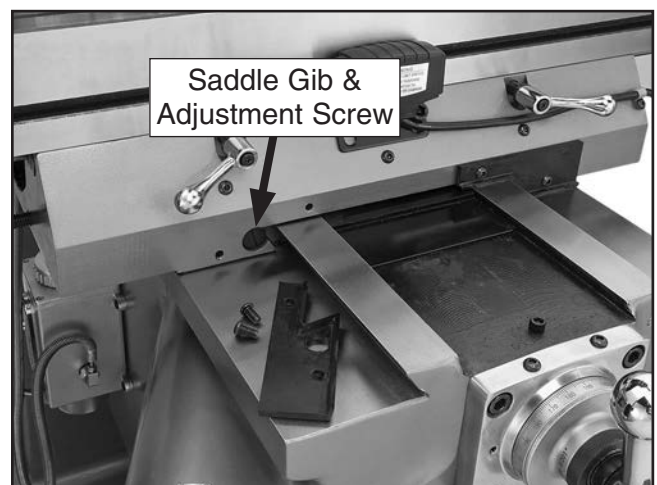
Figure 63. Saddle gib and adjustment screw.
