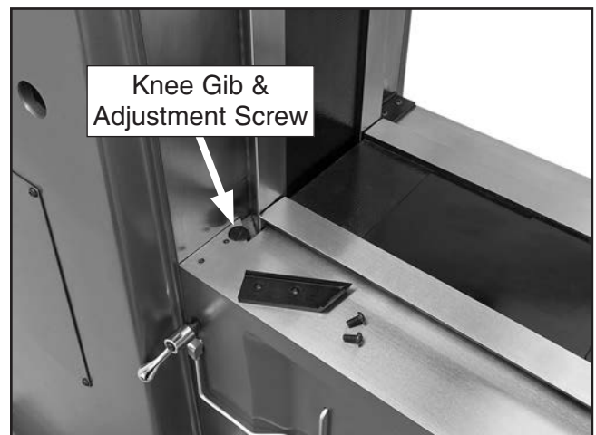
Figure 64. Knee gib and adjustment screw.
