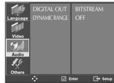
**2** Select a Digital Output. Set audio output to coaxial or optical. You can set the outgoing digital signal to BITSTREAM or LPCM:
