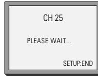
**3** If other stations are positioned on near the current RF OUTPUT CH, the guide message appears automatically.
