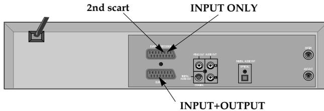
When connecting other equipment please refer to their manuals for further information. This video manual recommends the set up as shown on page 12. If the equipment is turned off when connected by this method, the video behaves as normal, but if the equipment is turned on the video will automatically switch over to AV2 mode and displays the channel of the other equipment, channel selection can only be performed by the other equipment, the video PR+ / PR- buttons have no effect.
