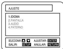
**2** Press the **Arrow** buttons (**▲/▼**) to select **DISPLAY** and then press the **ENTER** button.
