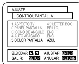
**4** Press the **Arrow** buttons (**▲/▼**) to select a desired item, and then press the **ENTER** button to change the setting.
