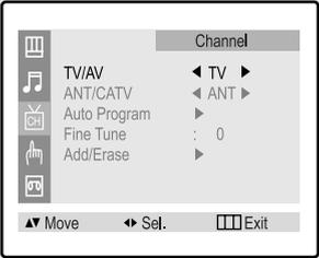
The screenshot shows a TV menu with the following items: TV/AV, ANT/CATV, Auto Program, Fine Tune, and Add/Erase. The 'Channel' option is highlighted. The 'Fine Tune' value is currently set to 0. Navigation icons for Move, Sel., and Exit are visible at the bottom.
