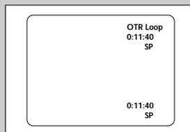
*One-Touch Recording (OTR) allows you to add recording time in 30-minute increments up to 9:30 minutes at the touch of a button.*
