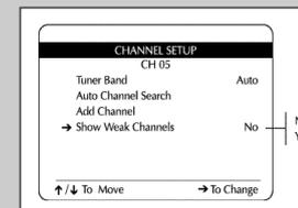
The "Show Weak Channels" feature allows you to view channels with weak reception rather than substitute a blue screen.
