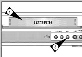
You can record a TV show in progress by inserting a blank tape and pressing the REC button. You can even add time in fixed 30-minute increments by pressing the REC button repeatedly; see page 50.
