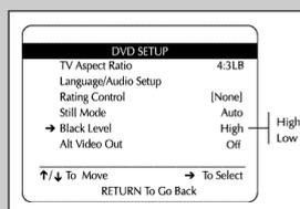
The Black Level feature adjusts the reference level of black in the video signal to one of two choices:
