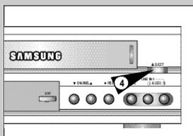
To play a videotape, simply insert it in the VHS deck and press the Play button. Tapes without Record Safety Tabs can be set to play automatically when inserted; see page 47.
