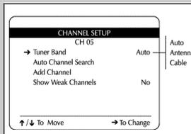
This feature allows you to manually set the DVD-VCR's tuner band to Antenna or Cable, whichever you connected to the Antenna In jack during initial setup.
