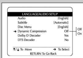
*Dynamic Compression constrains the dynamic range, i.e. the difference between the quietest and loudest passages of a DVD soundtrack. This enables you to limit loud noises, such as explosions, or raise the volume of quiet passages, such as whispering, while watching a movie. This is convenient for viewing movies late at night.*
