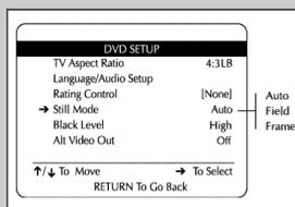
The Still Mode feature lets you set the default method of freezing a single image on the screen during DVD playback.
