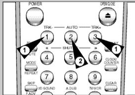
The Tracking adjustment removes the white lines that sometimes appear during playback because of slight differences in recording decks. The ATR button (Auto Tracking) will automatically align the recorded tracks with the playback heads to solve this problem. You may also set tracking manually.
