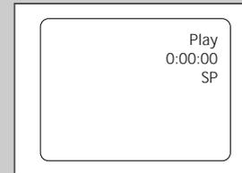
Press the DISPLAY button to see the current status of the VCR deck, as well as the tape counter position and record speed.
