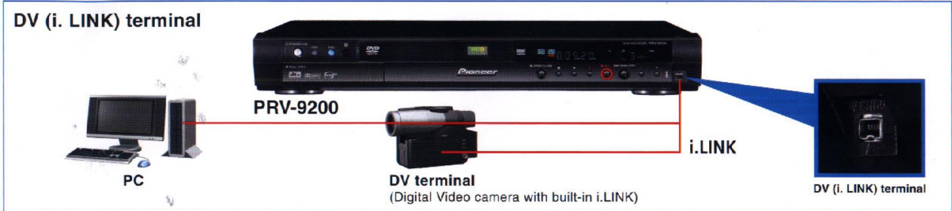
When recording from the DV input port in VR format, there is a limit on the transfer rate setting in order to maintain the highest video quality possible.
