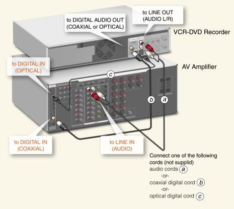
Connecting to an AV amplifier (receiver) with digital cords will enable you to listen to Dolby Digital or DTS surround effects. For further explanations, see "Connecting to Your AV/Amplifier (Receiver)" in the Operating Instructions.
