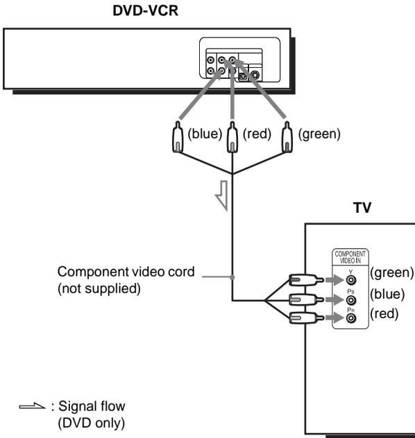
If your TV accepts progressive (480p) format signals, you must use this connection and then set “Progressive” to “On” in the “SCREEN SETUP” menu (page 69). The PROGRESSIVE indicator lights up in orange when the DVD player outputs progressive signals.
