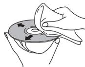
*Wipe lightly from the center of the disc using straight strokes.*
