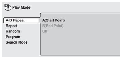
**3 Press ENTER on 'A(Start Point)' to set the loop start point.**
