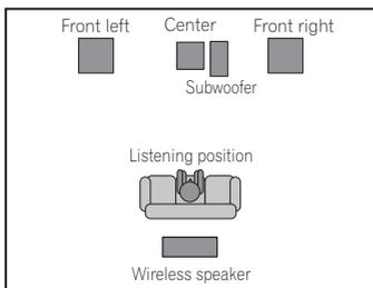
The following speaker placement options are only possible if you have connected a pair of speakers (not supplied) to the surround speaker terminals (refer to *Connecting the speakers and wireless speaker system* on page 12 to do this) and you are using the wireless speaker as a second stereo system (see *Using the wireless speaker system* on page 42 for more on this).
