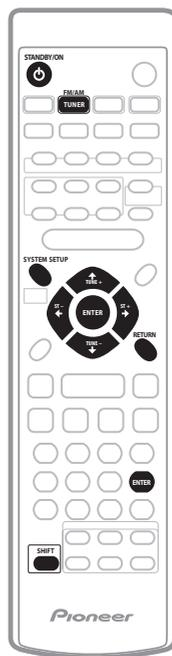
**1** If the system isn't already on, press
