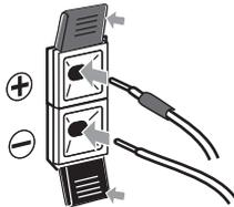
**3 Connect to the speaker terminals on the rear of the speakers in the same way.**
