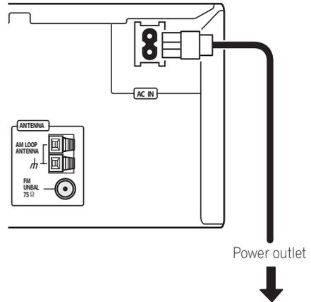
**1 Plug one end of the supplied power cord into the AC INLET.**
