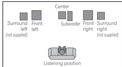
The surround speakers should be placed on either side of the front speakers and oriented either towards the walls, or straight ahead, depending on which mode you are using (see below).
