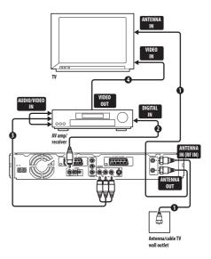
1 Connect RF antenna cables as shown.
