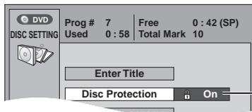
The lock symbol appears closed when the disc is write-protected.
