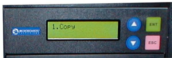
ENT button: The ENT button, used to start a duplication process or enter into an area in the menu structure.
