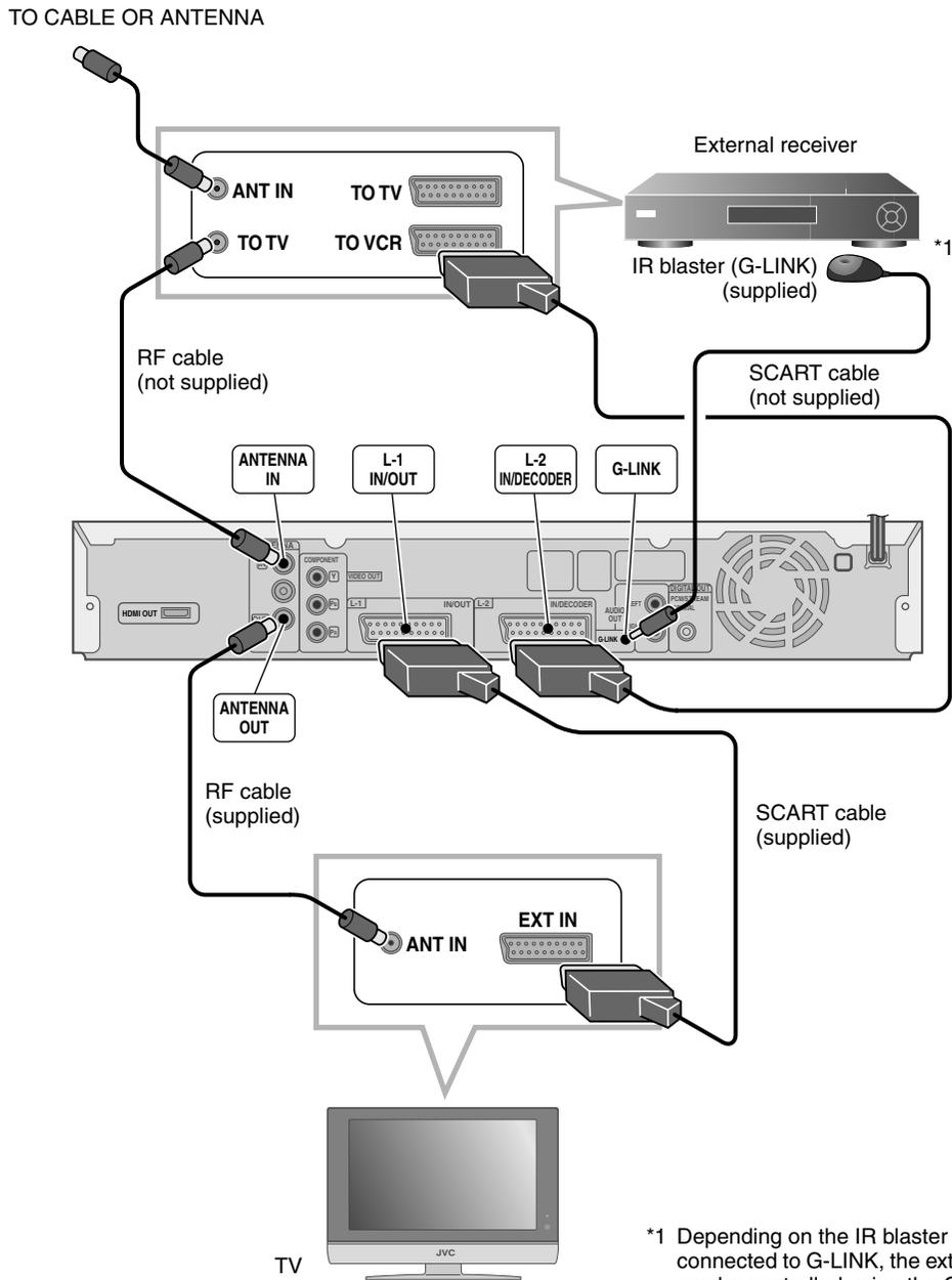
\*1 Depending on the IR blaster (G-LINK) connected to G-LINK, the external receiver can be controlled using the GUIDE Plus+ system. Do not place obstructions between the IR blaster (G-LINK) and the external receiver's infrared receptor.
