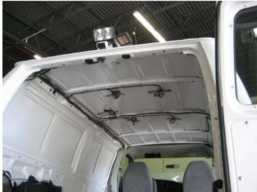
Be sure to tape harnesses to roof in approximate locations that accessories are being installed in Kwik kit. This will vary between the different model kits.
