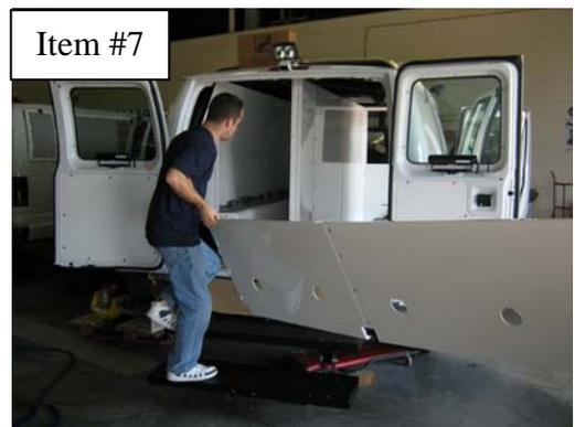
Loosely bolt **Center Divider** to **Front Bulkhead**
