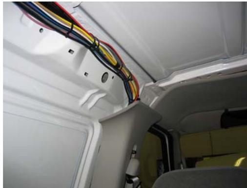
Run all wiring for dome lights, power vents, video system, HVAC, etc. at this time. Tie to existing OEM harness
