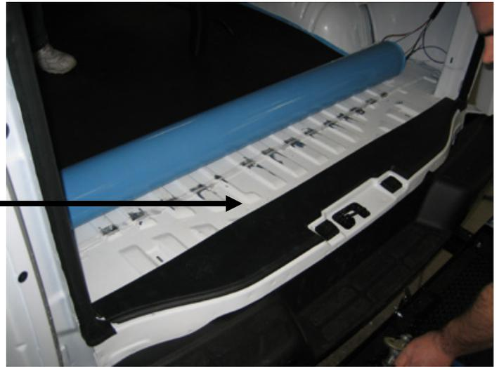
After plastic trim is cut and back in it's original location, you must measure 7" inches forward on both sides from newly cut trim to place rear Kwik Kit bulkhead. This is the starting position so parts fit into the correct locations. Note: With OEM rear AC/Heat, The kit will be shifted to passenger side.
