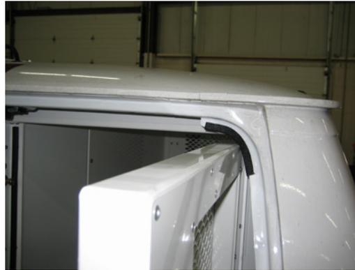
*Note: It is recommended to put edge molding on the OEM door opening on the passenger side to avoid damaging the Kwik kit door.*
