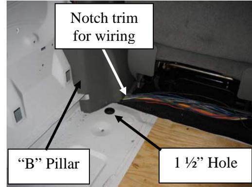
For neatness of wiring, route all cables down driver-side “B” pillar. If going under hood for power to console, drill hole at location above.
