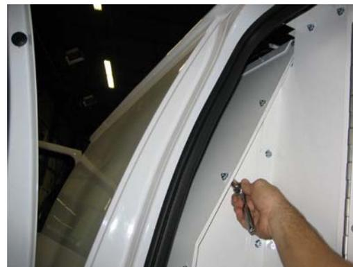
Begin to tighten **ALL** loose hardware on the remainder of the unit, being sure to align edges and bends of materials being tightened. This will square the unit to itself.
