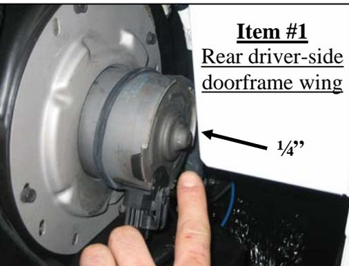
Position of driver-side **Rear Doorframe** when installing with factory rear air. *There should be at least 1/4" of space between the A/C blower motor and wing*
