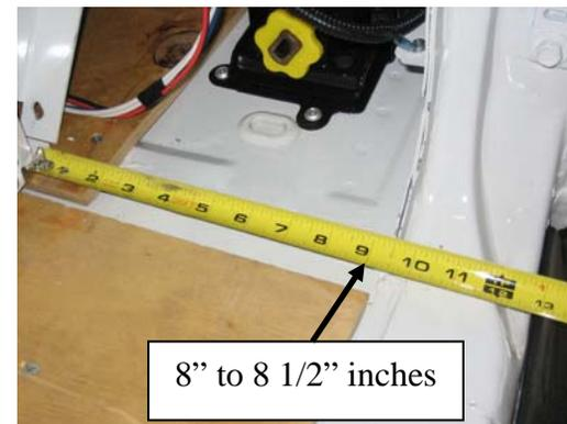
Measurement from passenger-side **Rear Doorframe** to vehicle doorframe shown above
