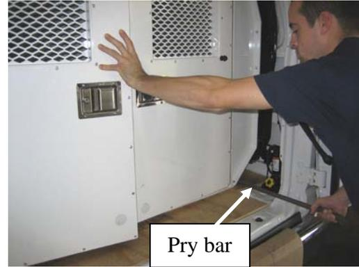
Position the entire unit according to the measurements on the following page. *Note: Maneuver the kit into position.*
