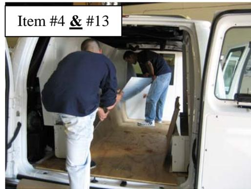
Be careful that exposed wires are not touching metal and optional **KK-x-VAK** hoses are not completely crushed
