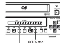
The setting value of the ENCODER QUALITY is indicated on the LCD display.
