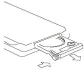
1. Press the catch and at the same time pull out the battery tray.
