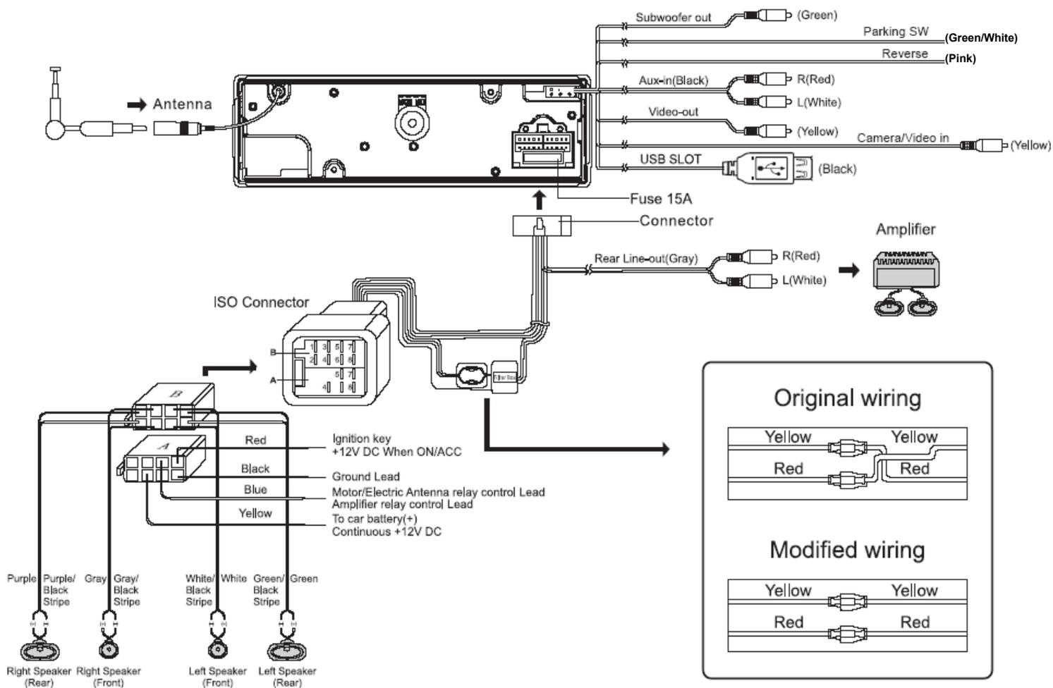
**Caution:** Do not interchange the connection of the wiring!!!
