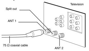
Connect to one of the terminals, then change the television's setting as necessary.
