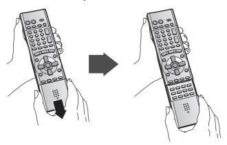
Hold both sides of the remote control's cover to open it. (You can also open it by pressing on the center of it and sliding it down.)
