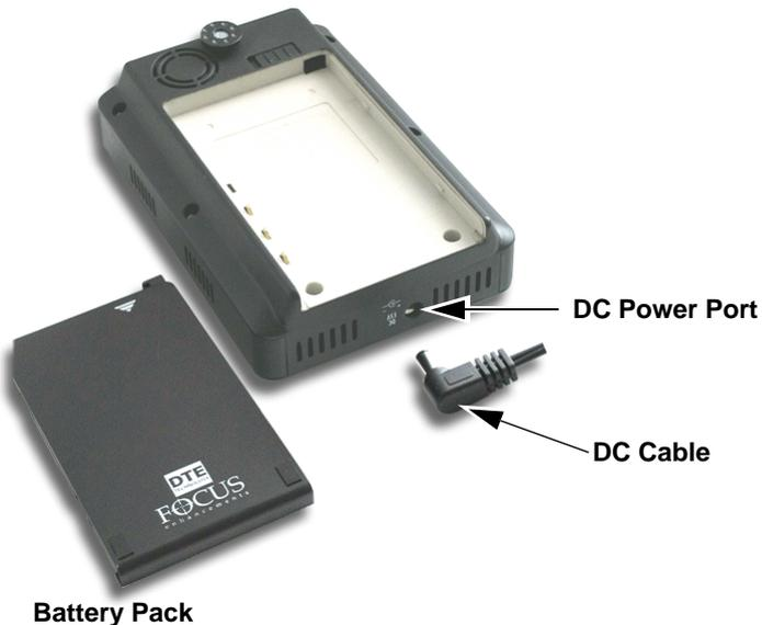
1. Plug the cord from the power supply into the bottom of the FS-4 HD.
