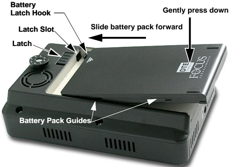
1. Place the unit, so that the battery compartment is up.
