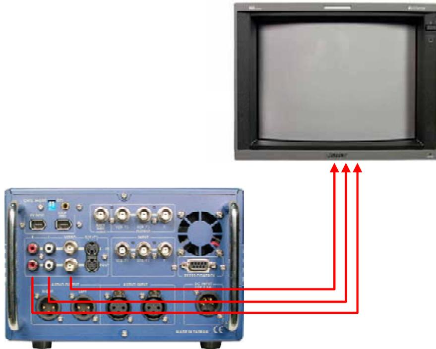
**2. Connecting YUV output from the MP-6000 to a Projector.**
