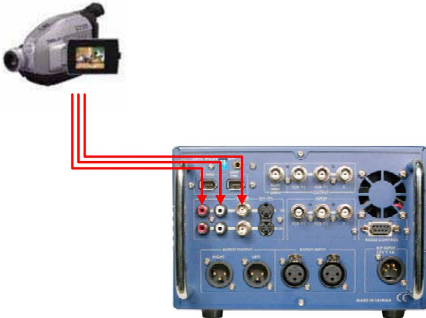
4. Connecting a DV (IEEE1394) output from a DV camcorder or DV Deck to the MP-6000. With this connectio
