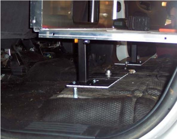
**Rear housing extension should be attached at this time**
