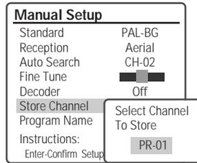
16 Use [▲/▼] to select 'Program Name'. Press [▶] to move to the second level. If your HDD/DVD Recorder is showing no station name or is showing a station name incorrectly, you can correct this.
