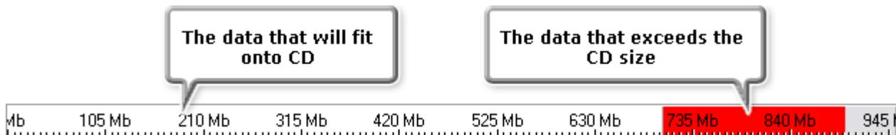
If the data size is greater than the capacity of a CD/DVD/BD you should either split your data into parts and record these parts onto several CDs/DVDs/BDs or select another disc type with a larger capacity. See the Appendix section for more information on different disc types.
