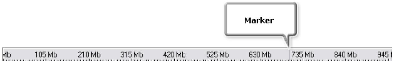
The Marker shows the standard capacity of a CD-R or a CD-RW - about 700 Megabytes.
