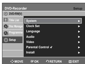
**3** Press the **▲▼** buttons to select **System**, then press the **OK** or **▶** button. System menu will be displayed.
