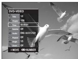
3 Enter the time in the sequence of hours, minutes, seconds using the number buttons, then press the **OK** button.
