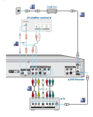
Connect the signal source to the STB or VCR Use a TV antenna or coaxial cable to connect the signal source coming from the antenna or wall to the VHF/UHF RF IN jack on the STB or VCR.
