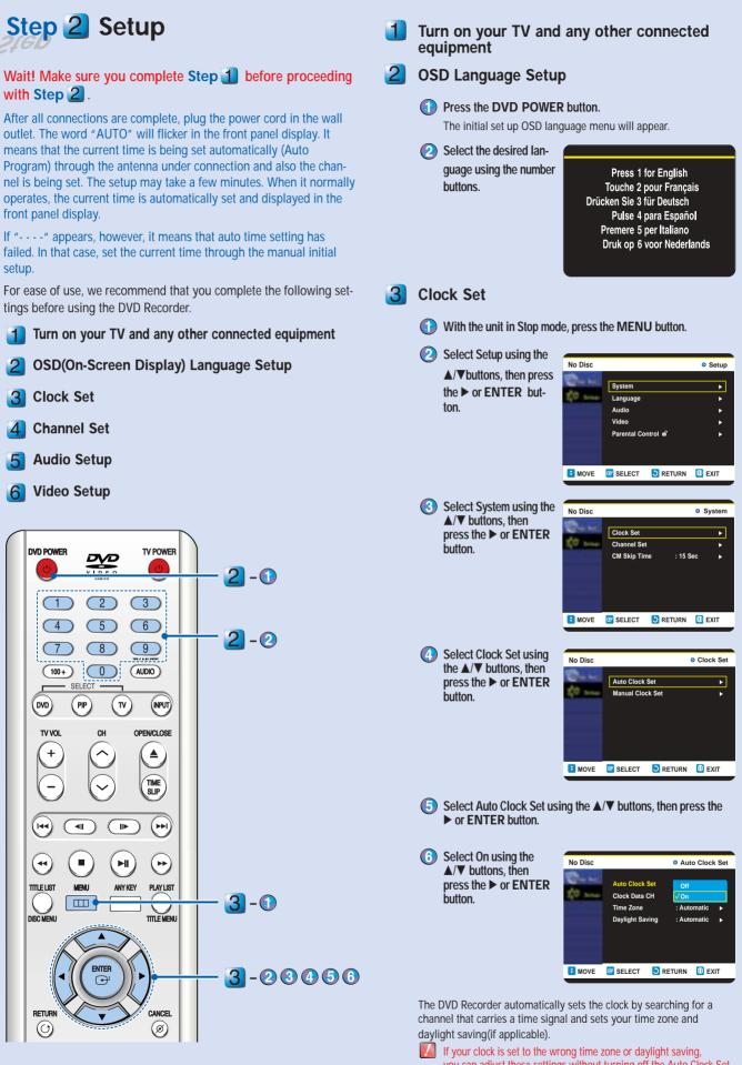
If your clock is set to the wrong time zone or daylight saving, you can adjust these settings without turning off the Auto Clock Set function (see page 24). If your clock cannot be set automatically, set the clock manually (Refer to "Manual Clock Set" on page 25 of the Instruction Manual for more information).
