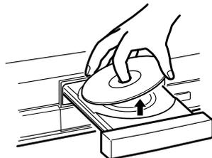
Be sure to press the **OPEN/CLOSE** button to close the disc tray after you remove the disc.
