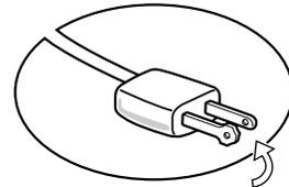
10. Protect the power cord from being walked on or pinched particularly at plugs, convenience receptacles, and the point where they exit from the apparatus.
