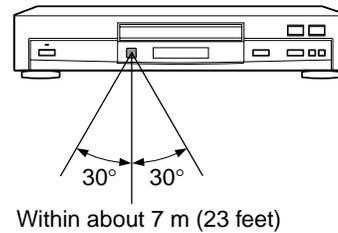
Distance: About 7 m (23 feet) from the front of the remote sensor
