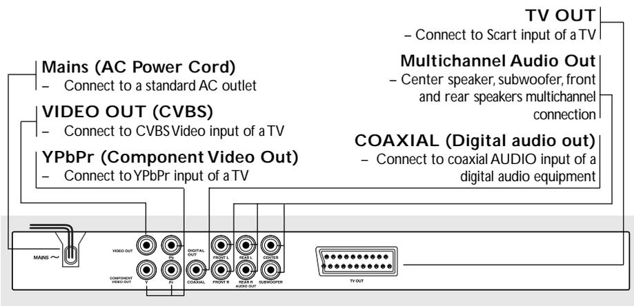
**Caution:** Do not touch the inner pins of the jacks on the rear panel. Electrostatic discharge may cause permanent damage to the unit.
