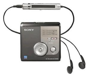
The HiMD recorders can record in two formats: the higher quality HiMD format or the Standard MD SP format. They can also record on both the old, "MD" discs and the new HiMD discs. The separate set-up steps for the Hi-MD mode follow these below.
