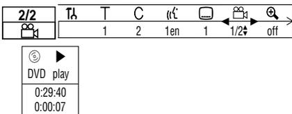
If the Angle symbol appears in the top left corner of the TV screen during play, multiple angles are available. Simply press **CH+▲** or **CH-▼** to switch among the different angles.
