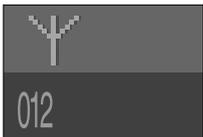
No signal - Channel is not receivable or no equipment is connected to the designated jack.
