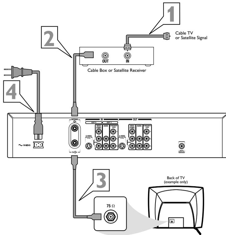
**1** Connect your Satellite or Cable TV signal to the **ANTENNA IN** jack on your Cable Box/Satellite Receiver.
