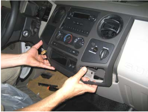
Carefully detach upper dash panel assembly from spring clips.
