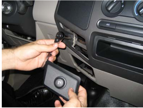
Carefully remove the small dash panel that holds the lighter plug. Use 7mm socket and remove dash mount screw
