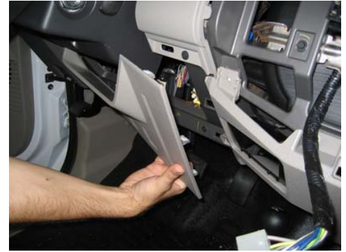
Detach lower dash panel under steering column.
