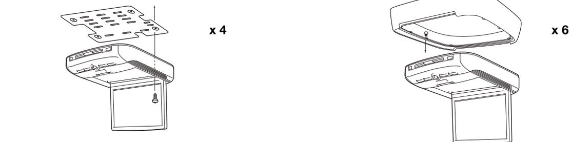
\*1 Installation Bracket is used to stabilize the monitor at the time of installing the monitor. Ask ALPINE dealer for detail.
