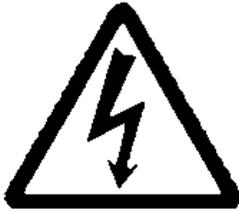
**Warning!** — This symbol alerts you to a potentially hazardous condition, such as the presence of dangerous voltage that could pose a risk of electrical shock. Refer to the accompanying Warning Label or Tag, and exercise extreme caution.
